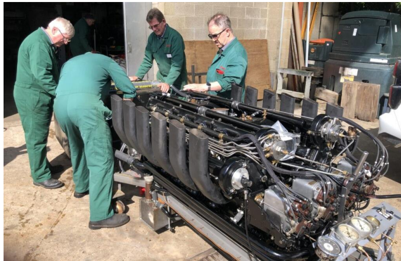
One of the two Sunbeam 22.5 litre V12 Matabele aero engines recently under restoration at Beaulieu. The rear engine air starting system gauges can be seen on the RHS
