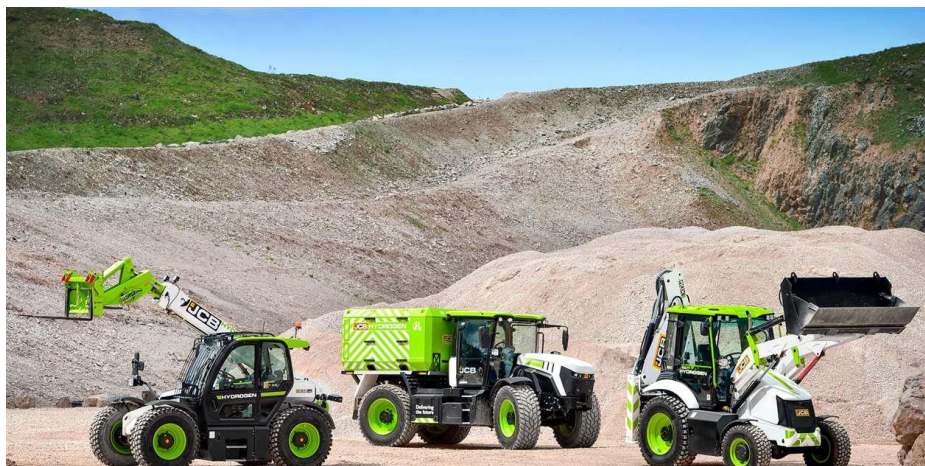
The current JCB Hydrogen powered range with the Fuel Bowser shown centre
