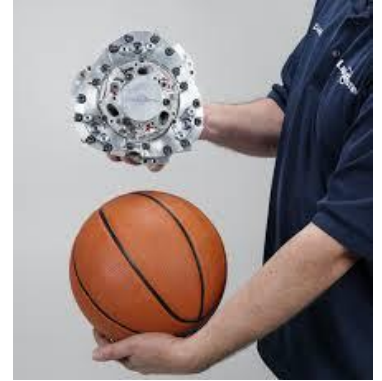
The 2 stroke 25hp liquid cooled, naturally aspirated 210cc Liquid Piston engine.
