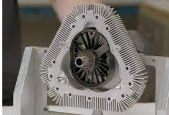
The 2 stroke 25hp liquid cooled, naturally aspirated 210cc Liquid Piston engine.
