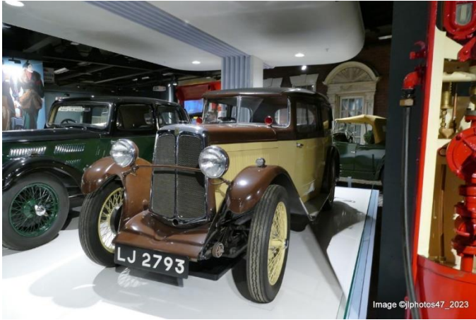
1930 Standard Swallow. This used a Chassis made by the Standard Company and coachwork by SS Cars Ltd.
