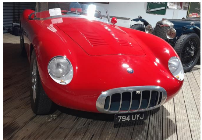
1956 OSCA MT4 1.5 litre, 110 hp twin cam engine
